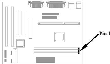
The DIMM types supported are EDO (Extended Data Out) and SDRAM (Synchronous DRAM). This mainboard has three 168 pin DIMM sockets (Dual-in-line Memory Module) that allow you to install system memory up to **256MB**.
