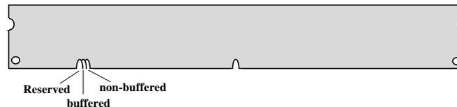
Because the positions are different, only non-buffered DIMMs can be inserted into the DIMM sockets on this motherboard. Although most of DIMMs on current market are non-buffered, we still recommend you to ask your dealer for the correct type.
